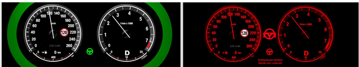
Figure 5-1: Improved HMI concept with more prominent color display when L2 is activated compared to the HMI concept of Study 2 (green frame; left) and when warnings are displayed (red filling; right)
