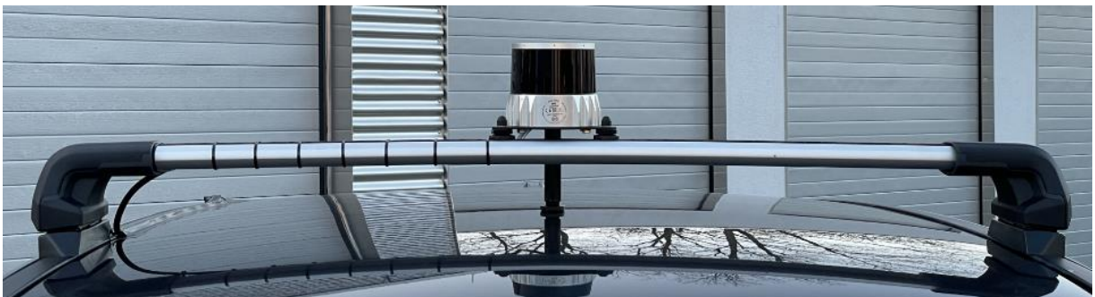
Figure 4-8: LiDAR sensor installation on roof rack (BMW iX)
