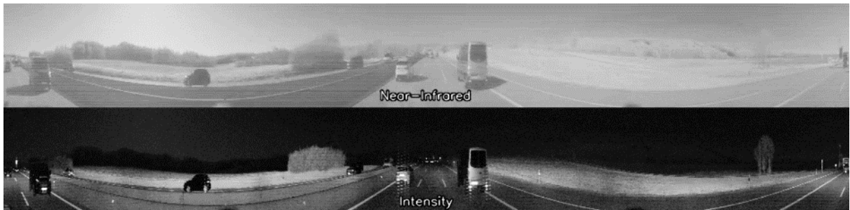
Figure 4-9: 360-degree image representation of LiDAR point cloud data
