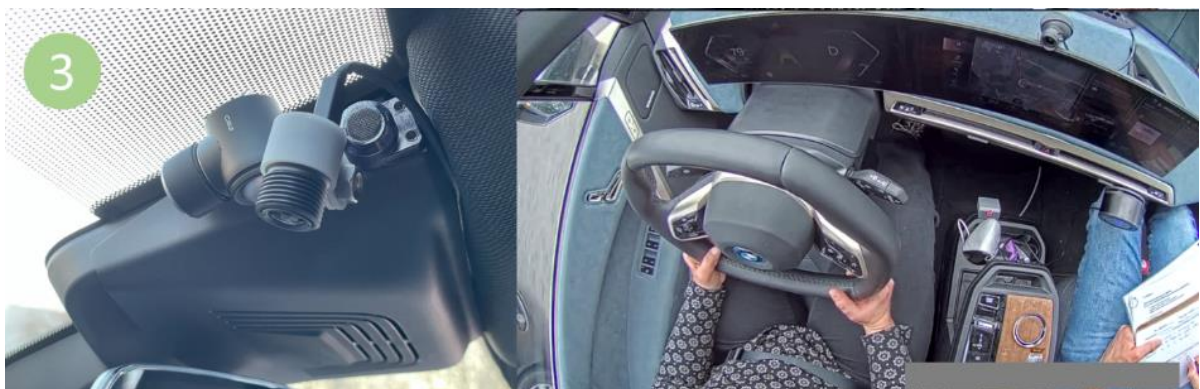
Figure 4-6: Exemplary camera sensor placement of Steering Wheel camera (BMW iX)
