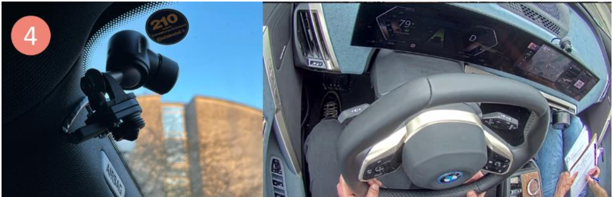
Figure 4-7: Exemplary camera sensor placement of Instrument Cluster camera (BMW iX)
