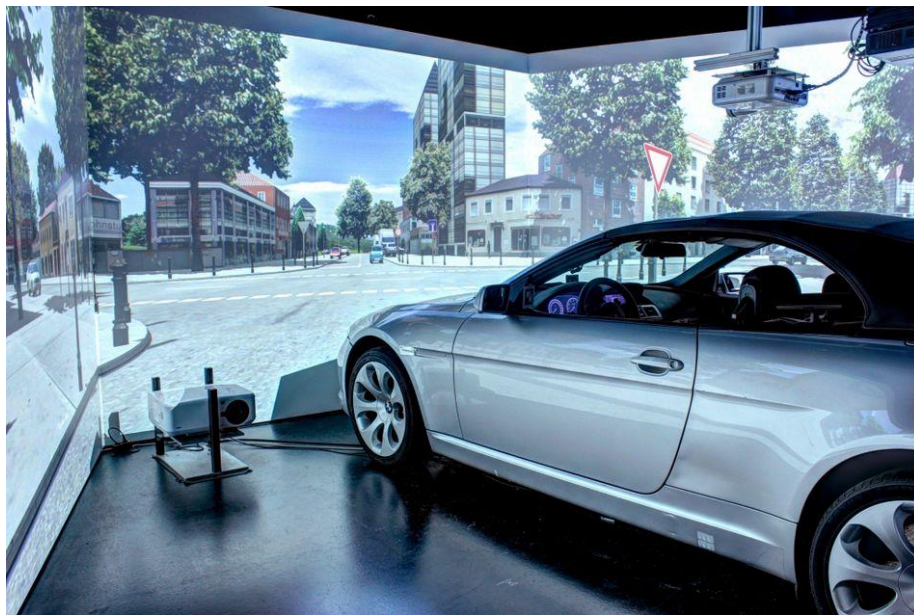
Figure 5-6: Static driving simulator of the Chair of Ergonomics at the Technical University of Munich.
