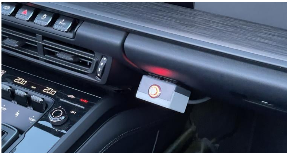
Figure 4-11: Trigger button for marking of special situations (Porsche 911)
