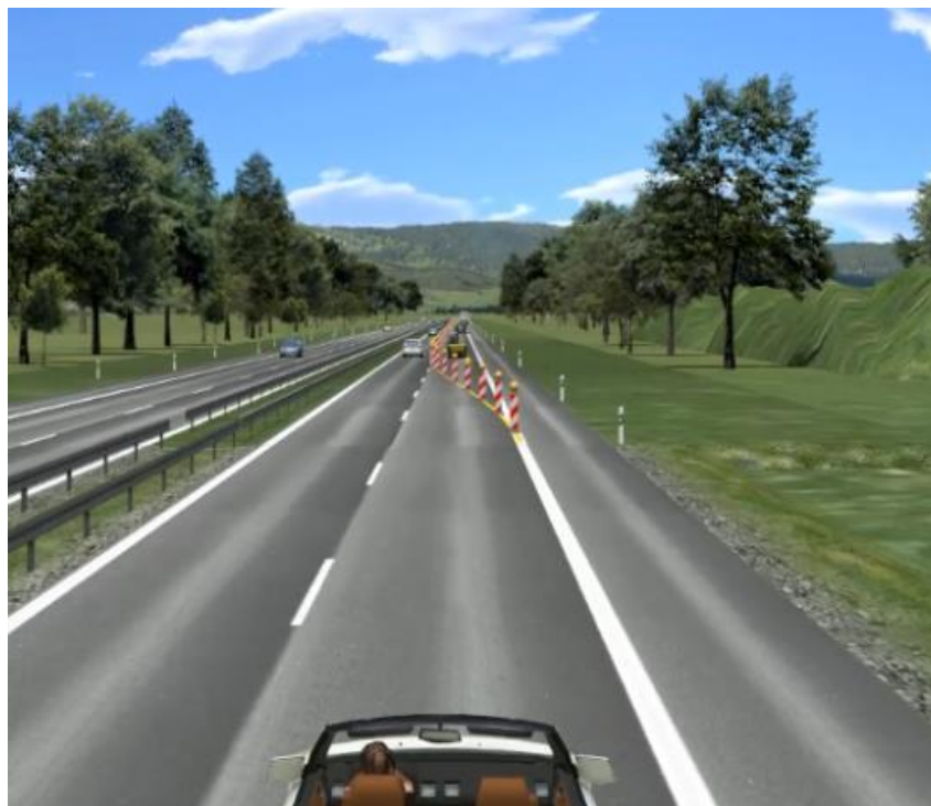
Figure 5-10: Visualization of Scenario 2 (system limit caused by roadworks blocking the right lane)
