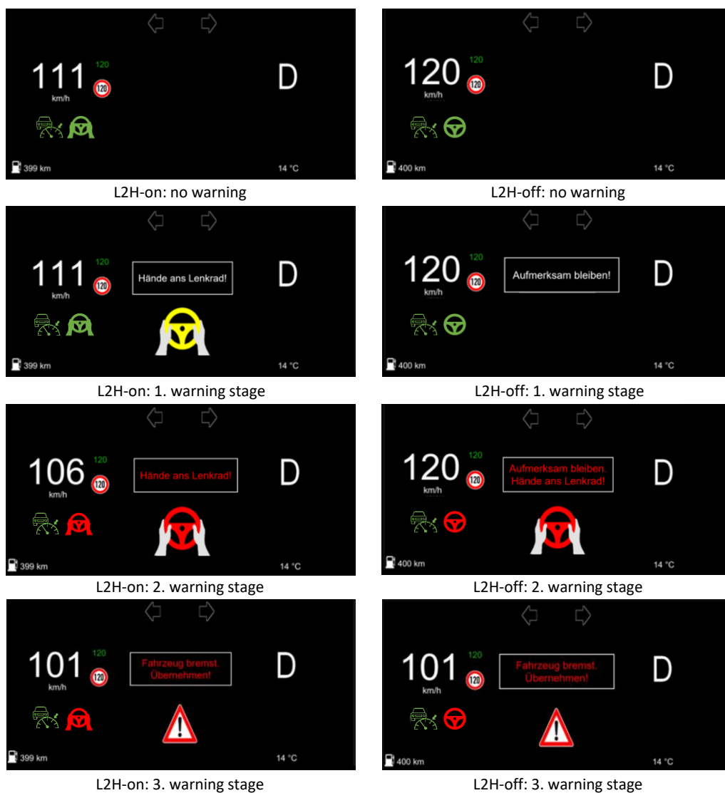
Figure 5-8: HMI design of the L2H-on function (left) and the L2H-off function (right) for L2-driving without any warnings and the three warning stages
