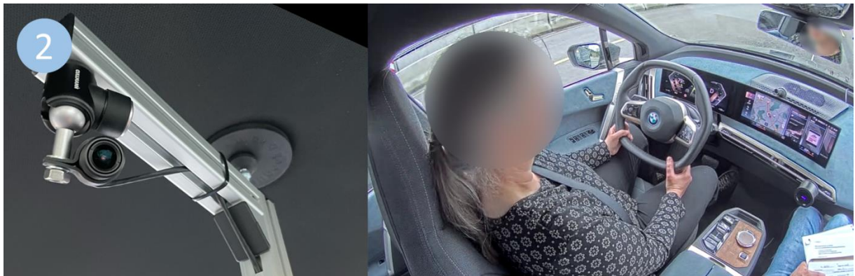
Figure 4-5: Exemplary camera sensor placement of Body Pose camera (BMW iX)
