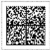
Module size is determined automatically (i.e. the entire 18 x 18 mm area is used)
