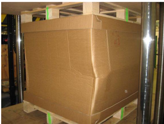
Determining the breaking load of a corrugated GLT.
