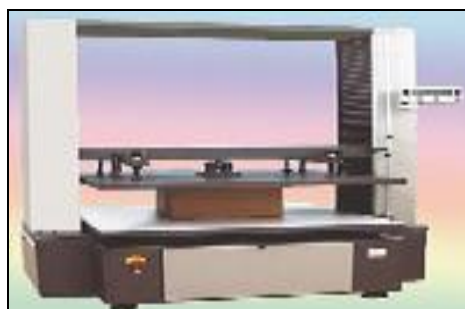
Figure 15: Box Compression Test (BCT)
