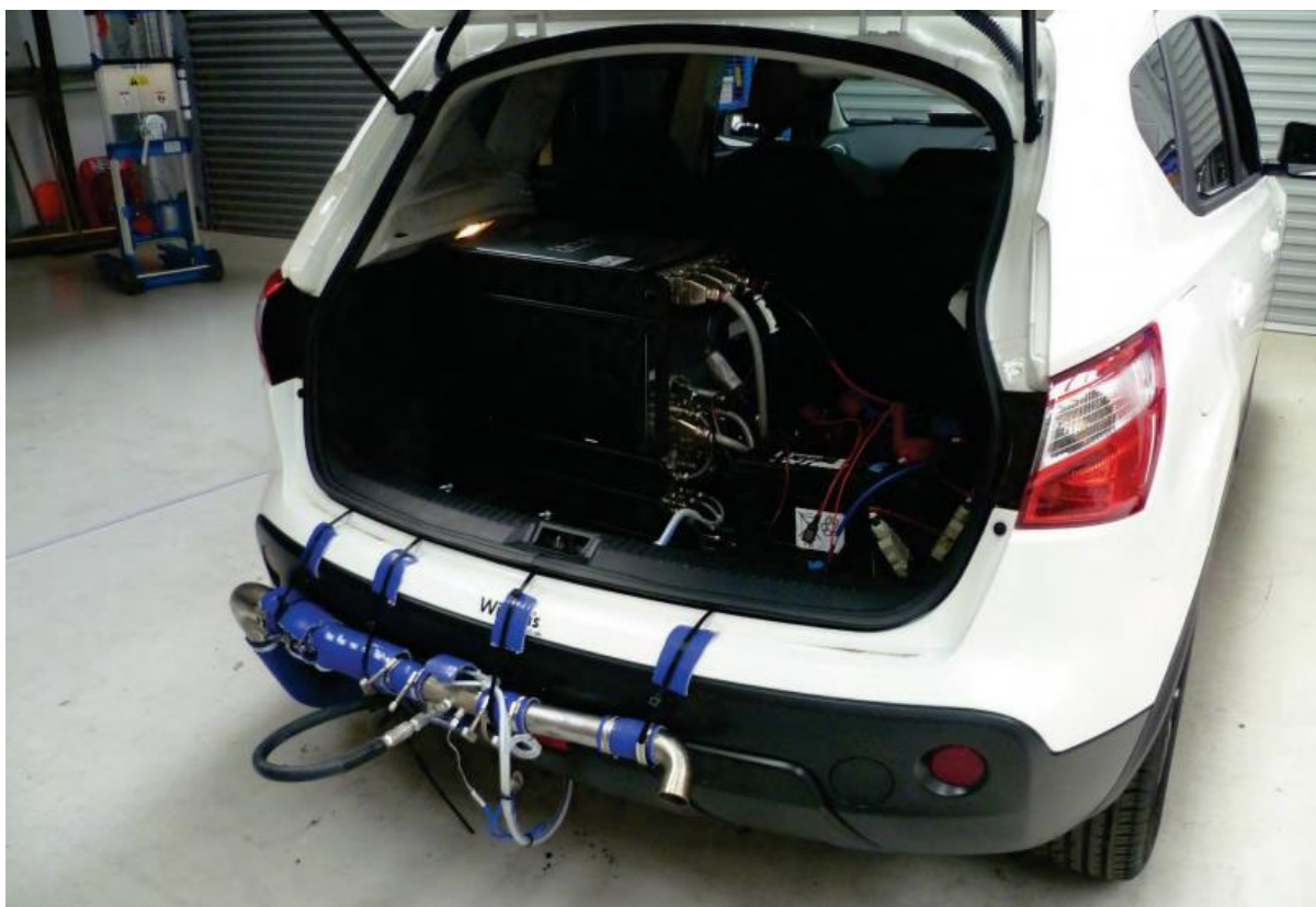
Figure 9 PEMS within a test vehicle, as used in The UK Department for Transport (2016) (Figure 4-1, The UK Department for Transport (2016))
