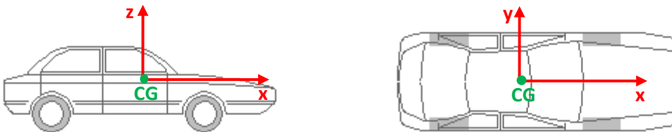
Figure 4.4 – Local coordinate system of GIDAS based PCM
