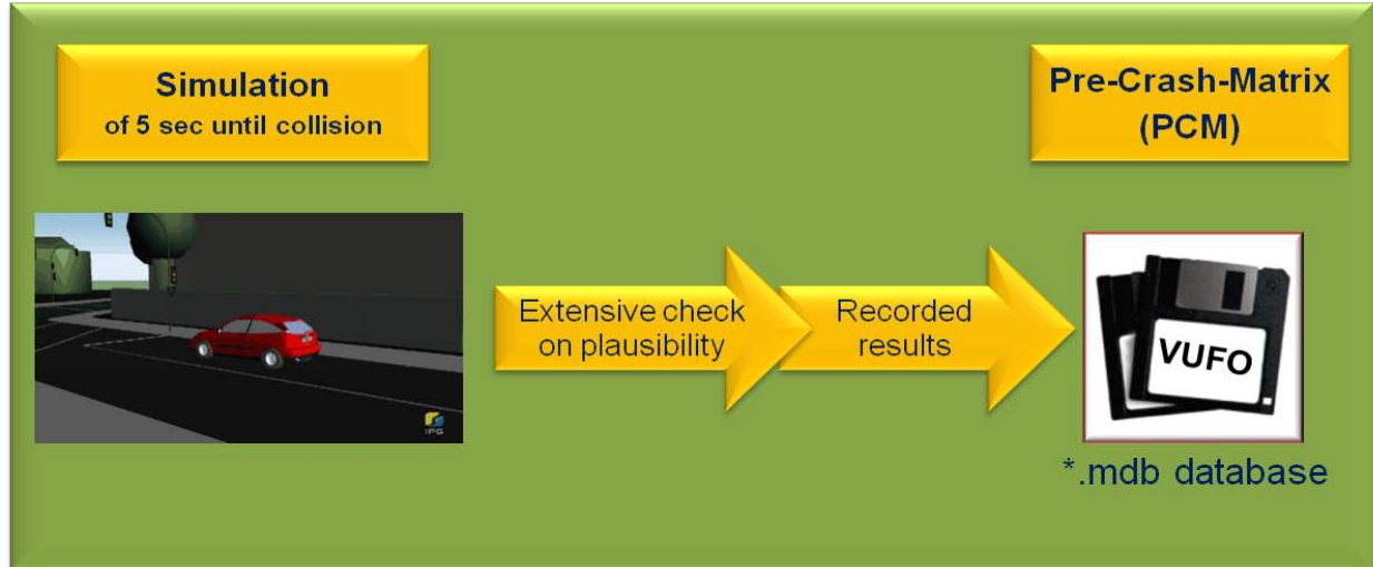
Figure 2.4 – Process of PCM creation on the basis of GIDAS
