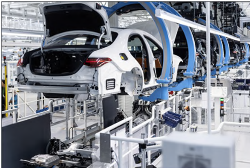
Flexible marriage – a new interpretation to a classic work step Fullflex Marriage in Factory 56 of Mercedes-Benz AG in Sindelfingen (source: Mercedes-Benz AG)
