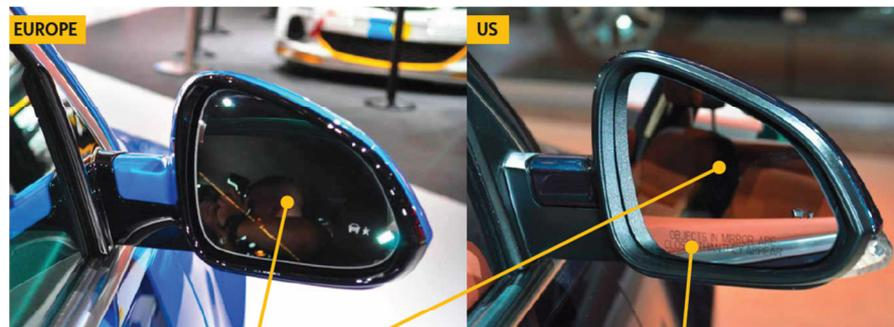
Different optical properties (curvature of the mirror)
