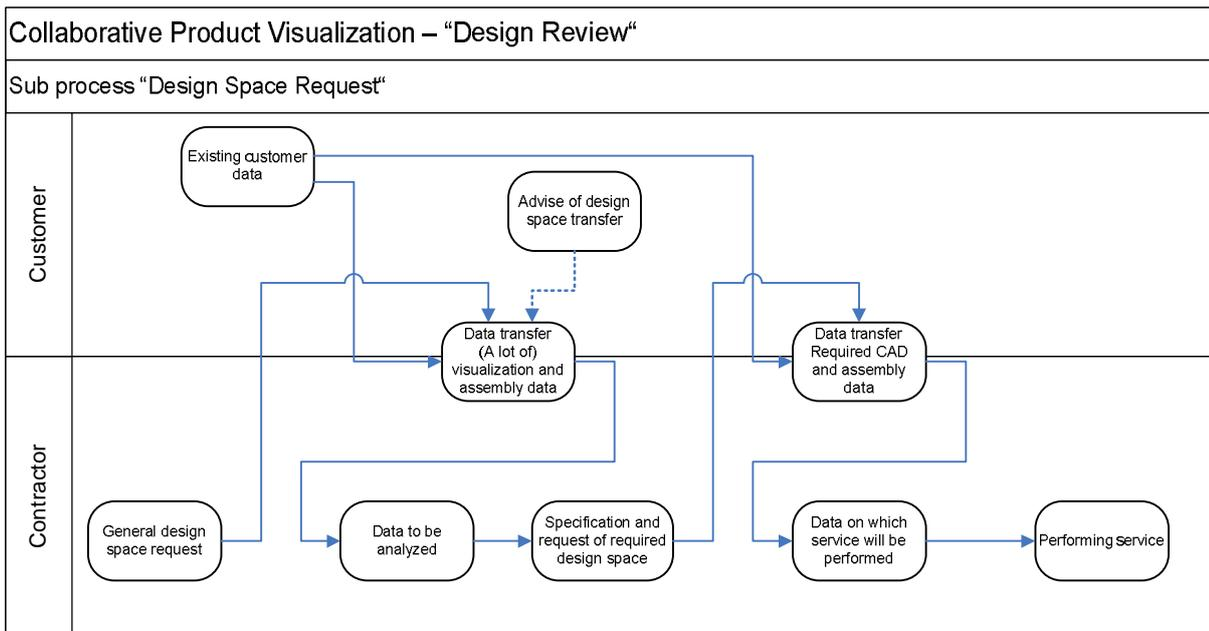
Figure 4 Process diagram “Design Space Request”
